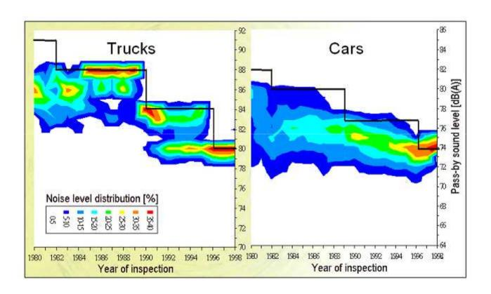
Development mean noise levels during type approval testing, NL
