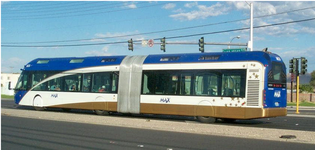
Figure 3. Civis diesel-electric hybrid bus
